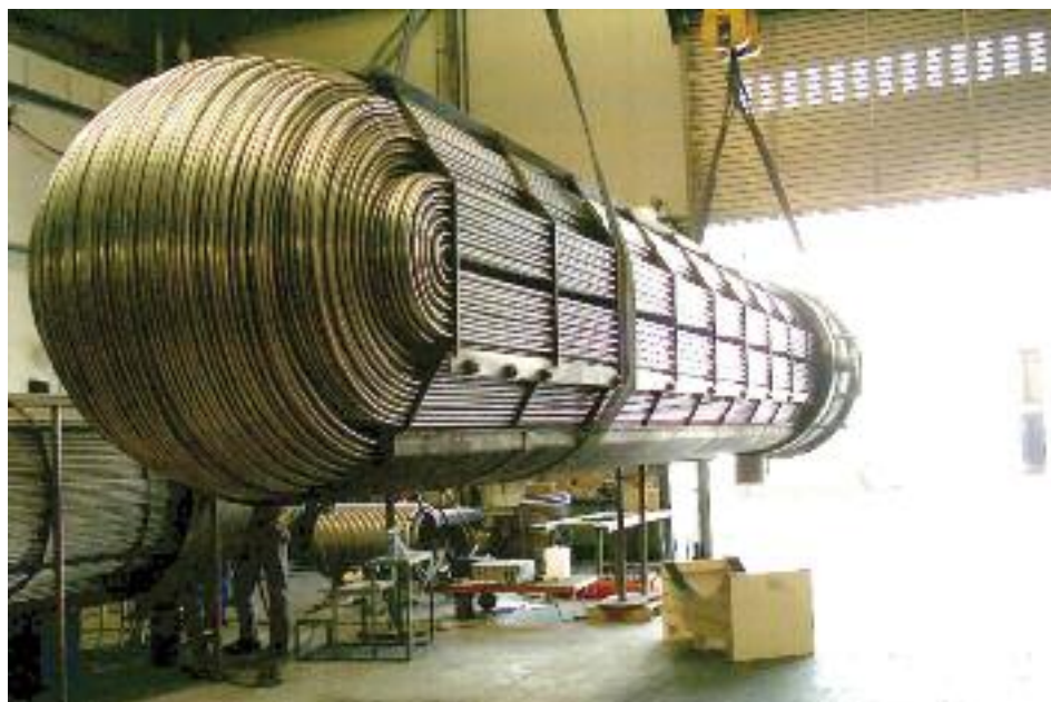
Industrial scale heat exchanger
